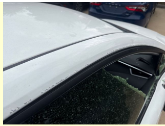
Right drip rail mult dents/paint dam
