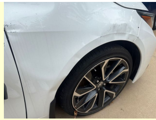
Rf fender mult dents/paint dam
