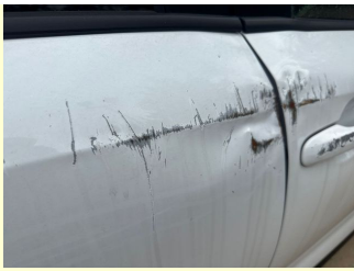
Rr door severe damage
