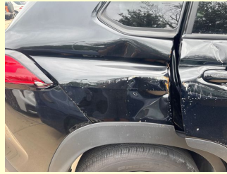
R qtr panel severe damage
