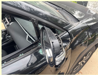
Rf mirror severe damage
