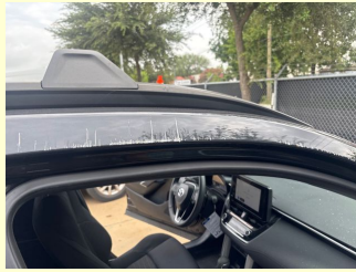
Right drip rail scratch heavy
